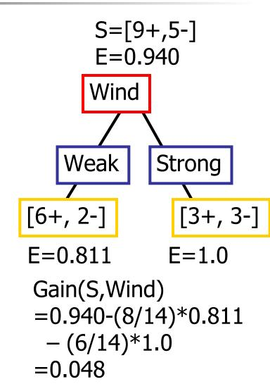
Humidity provides greater info. gain than Wind, w.r.t target classification.
