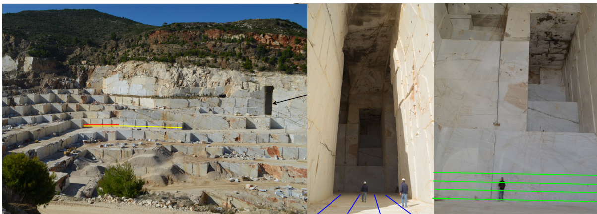
Figure 3 Dionyssos-Pentelikon. S.A. quarry (left) with the underground chamber (center and right). Yellow, blue and green lines denote GPR profiles while the red denotes the ERT profile.
