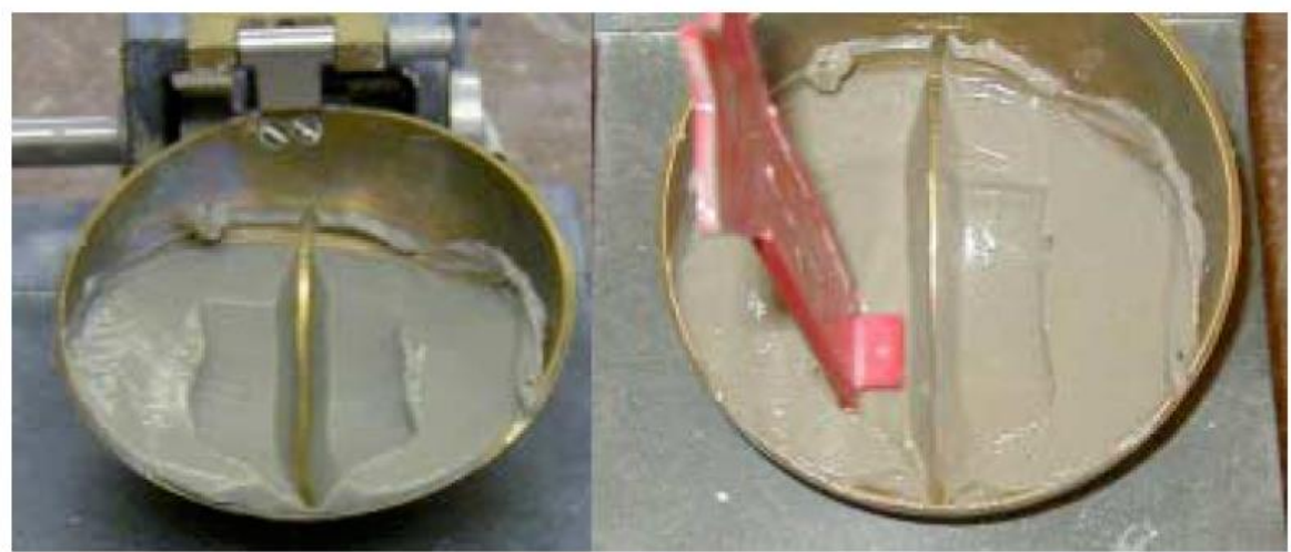
Figure 3 - Left, groove separating two halves of pat, right, stop blow counts after this length of groove closes a length of 13 cm.
